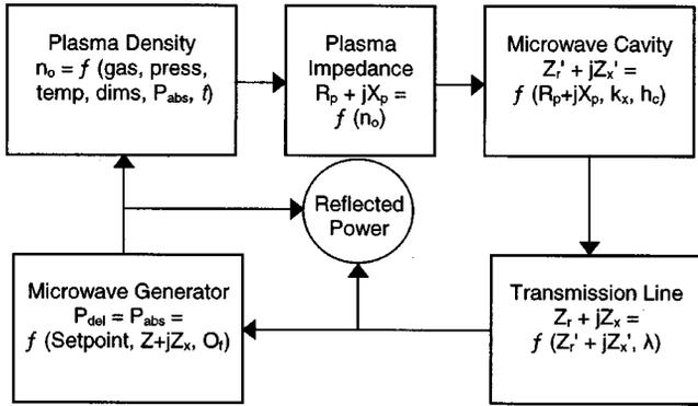
FIG. 4. Plasma system model block diagram.
