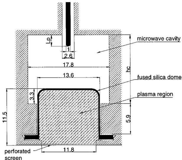
FIG. 2. MCPR with all dimensions in centimeters.
